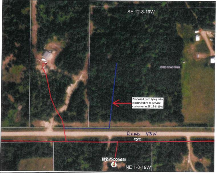
Offset of Fibre distribution and Handhole Vaults are 3m (unless otherwise specified) from adjacent property line within ROW Hand hole Vaults are 2 ft by 3ft and are flush with ground level.
