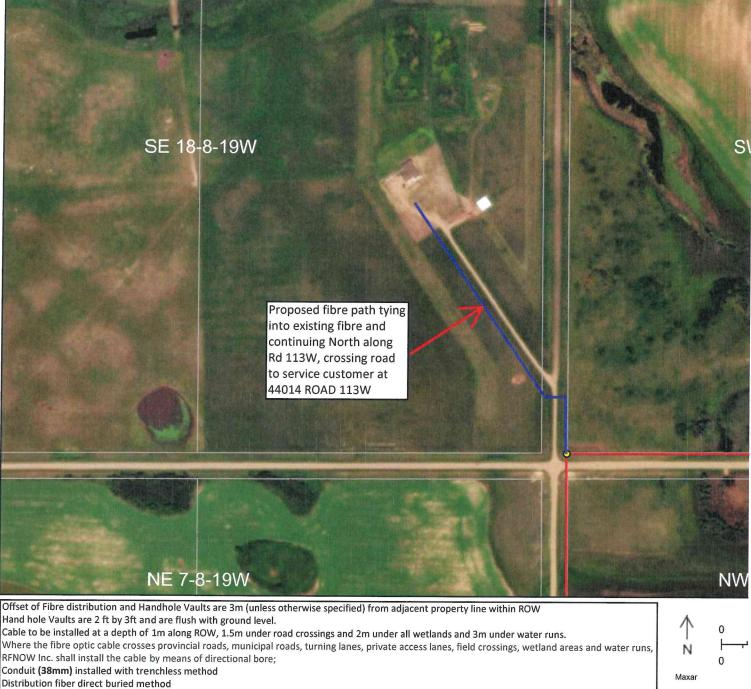
1m separation vertical or horizontal around existing underground utilities.
